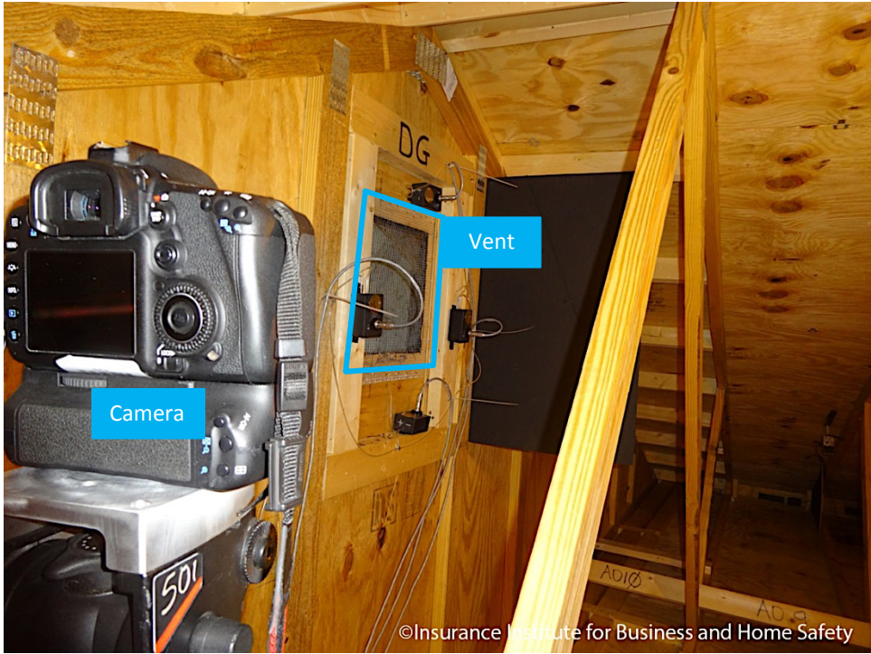
Figure 11. Typical video camera setup used to evaluate ember entry through the gable end vent.
