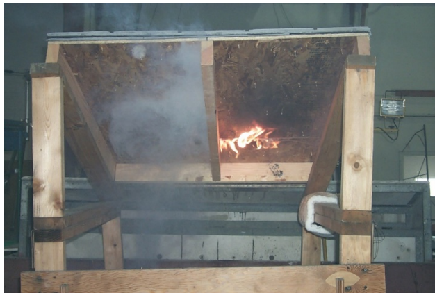
Figure 3.1. During a standard test to determine the fire rating of a roof covering. For this test, a Class A burning brand (wooden crib) was placed on top of the roof covering. Flames on the underside of the roof indicate that, as constructed, this roof covering is not Class A. Photo: Stephen L. Quarles
