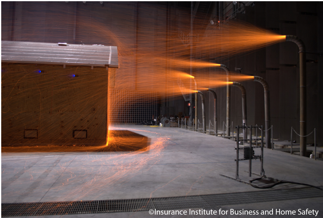
Figure 10. Ember generators operating during a test.
